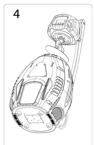
1. Lay the fixture on its' back and remove the two Phillips screws labeled "A" and "B" found on the bottom plate of the fixture.
