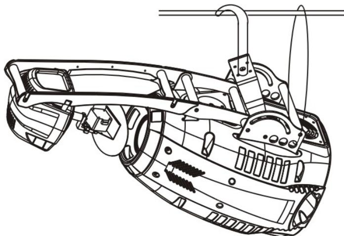
Screw one clamp each via a M10 screw and nut directly into the bracket of the scanner. Pull the safety-chain through the bracket of the base and over the trussing system or a safe fixation spot.
