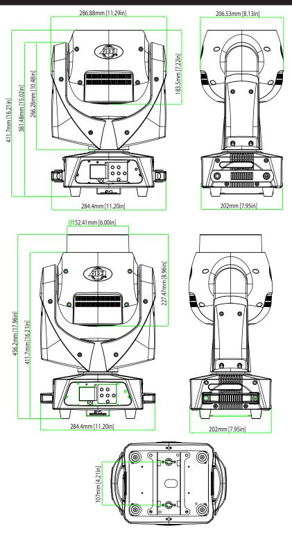
When installing the unit, the trussing or area of installation must be able to hold 10 times the weight without any deformation. When installing the unit must be secured with a Secondary safety attachment, e.g. and appropriate safety cable. Never stand directly below the unit when mounting, removing, or servicing the unit.
