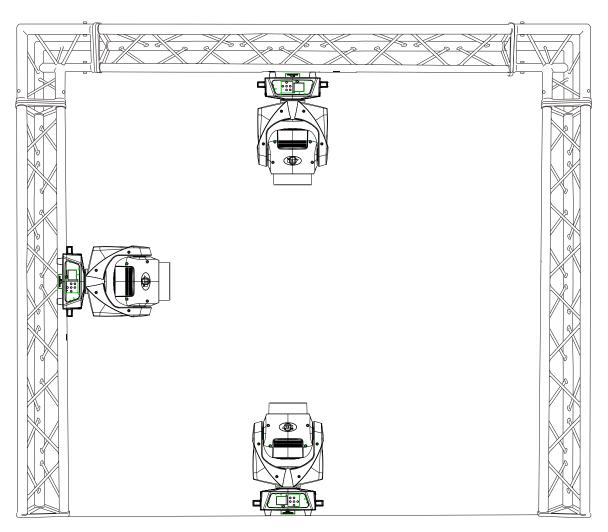
The Vizi Hex Wash7 is fully operational in three different mounting positions; hanging upside-down from a ceiling, mounted sideways on trussing, or set on a flat level surface. Be sure this fixture is kept at least 0.5m away from any flammable materials (decoration etc.). Always use and install the supplied safety cable as a safety measure to prevent accidental damage and/or injury in the event the clamp fails (see next page). Never use the carrying handles for Secondary attachment.
