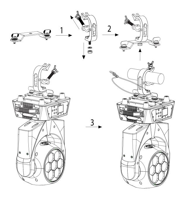
Screw one clamp each via a M12 screw and nut onto the Omega holders. Insert the quick-lock fasteners of the Omega holders into the respective holes on the bottom of the Vizi Hex Wash7. Tighten the quick-lock fasteners fully clockwise. Install the second Omega holder. Pull the safety-cable through the holes on the bottom of the base and over the trussing system or a safe fixation spot. Insert the end in the carabiner and tighten the safety screw.
