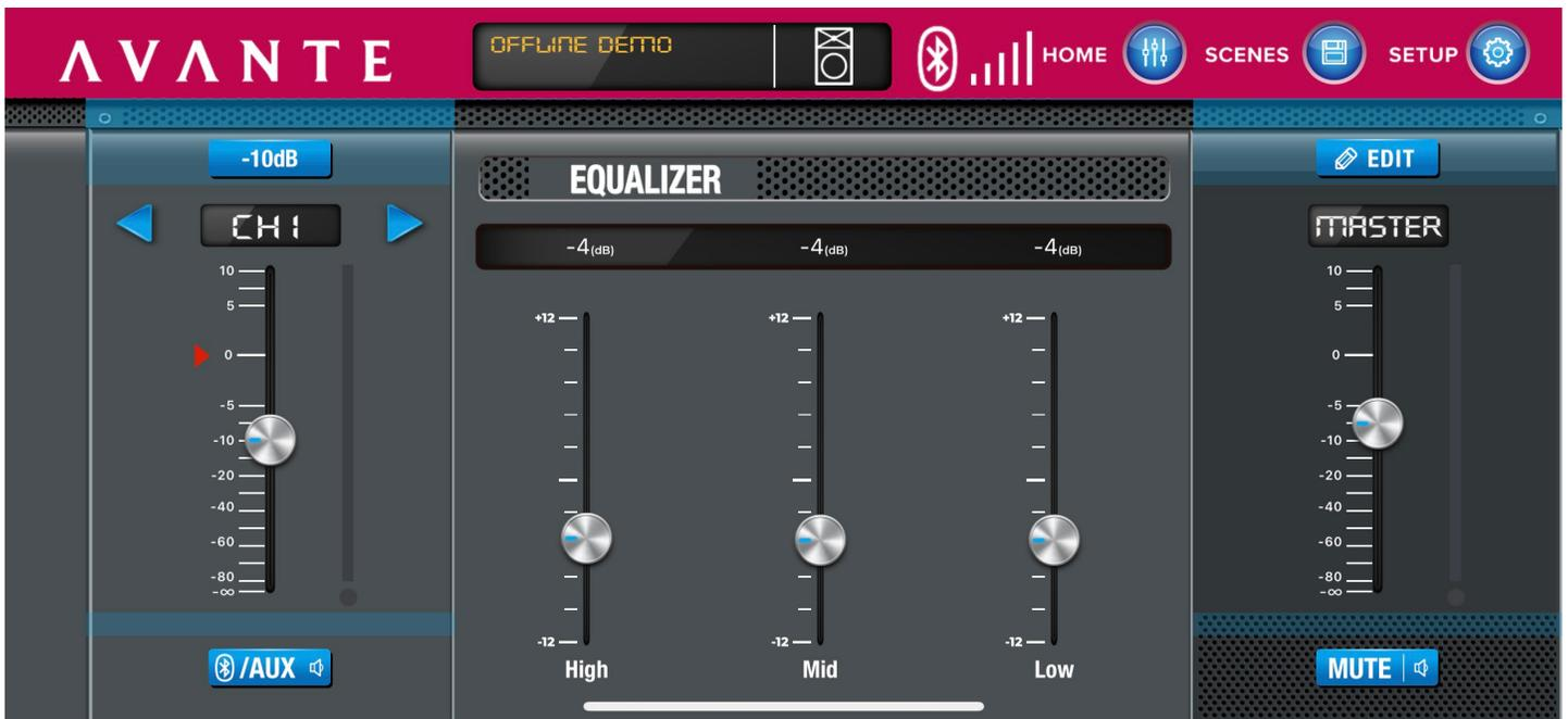
**Channel 1 Page:** adjust the volume and EQ of Channel 1. Note that the Master Volume can also be adjusted here.
