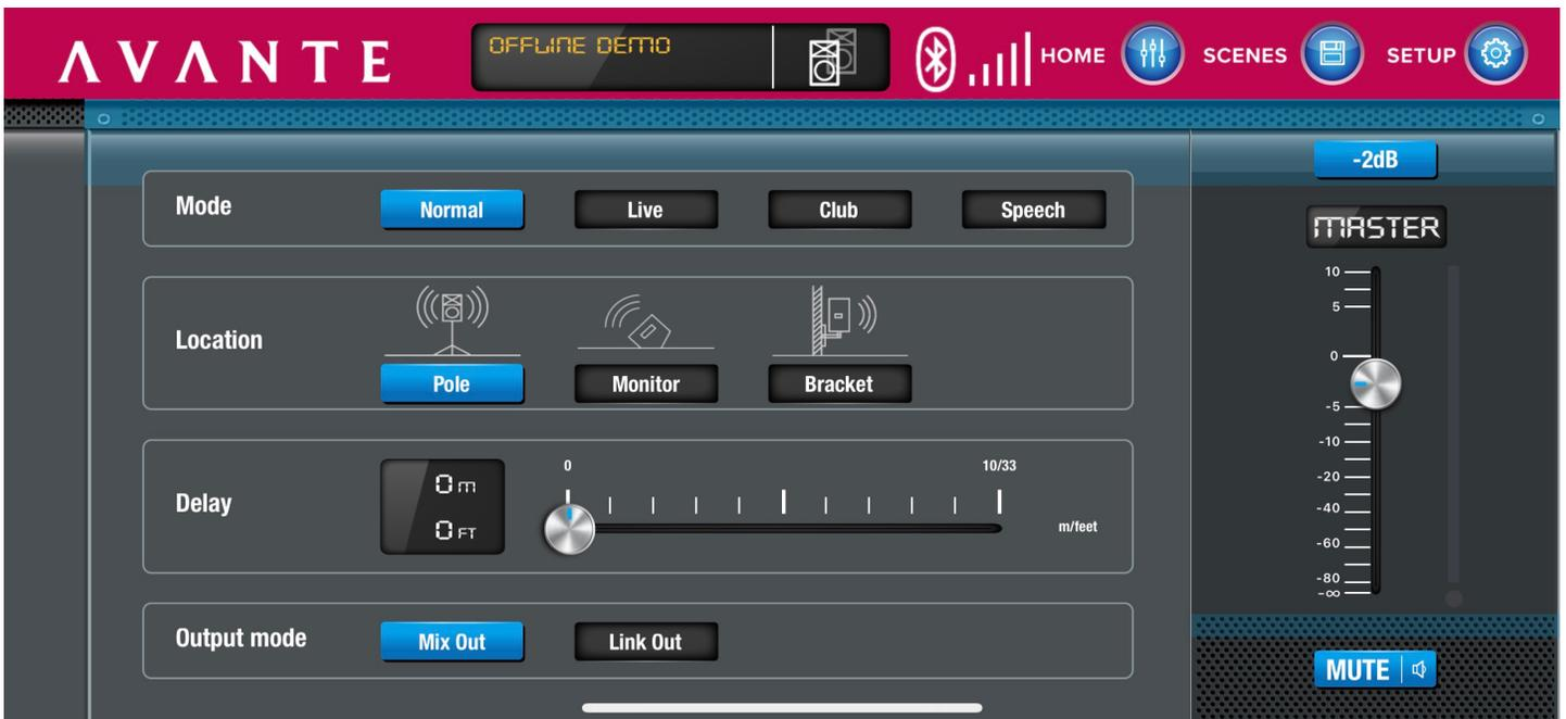
**Master Channel Page:** adjust the volume, mode, Location, delay, and output mode of 2 channels.
