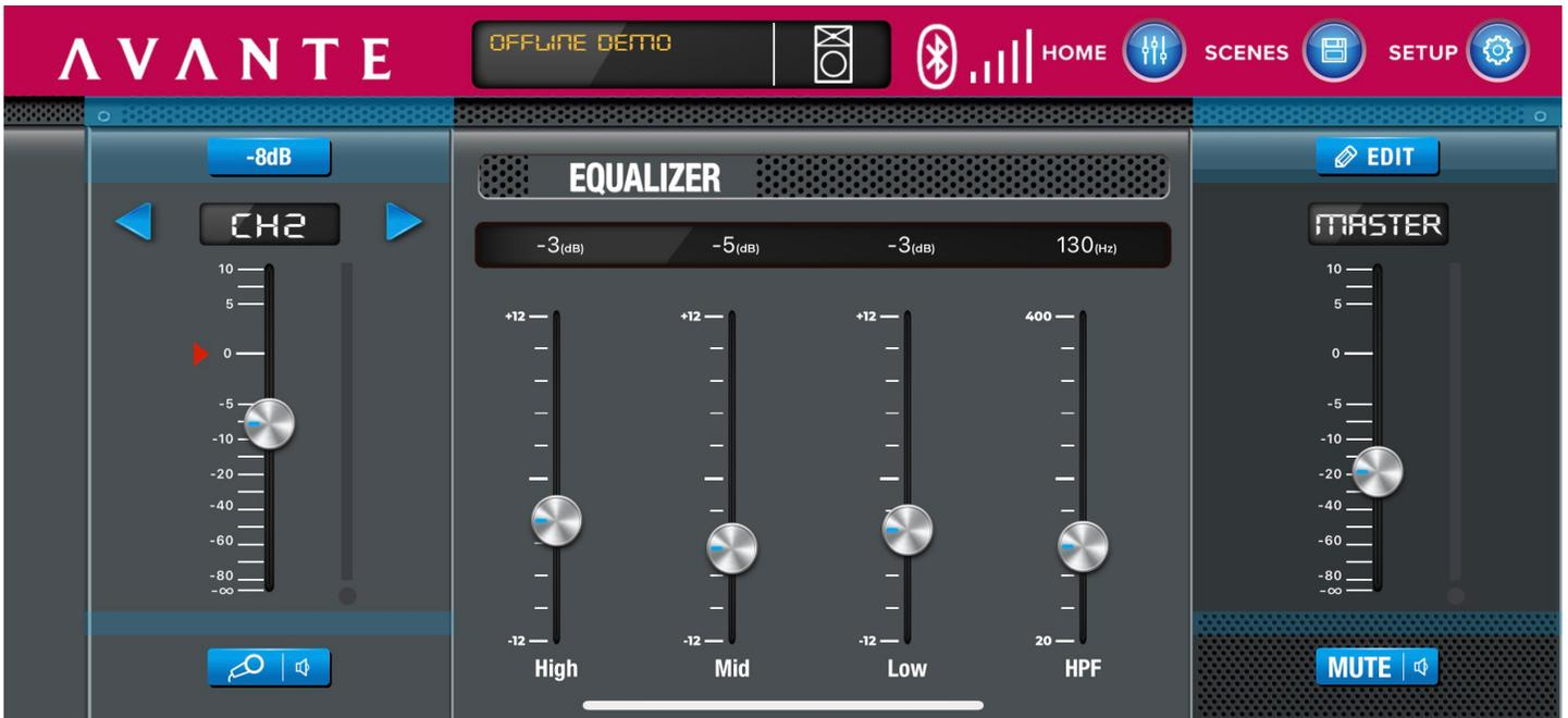
**Channel 2 Page:** adjust the volume and EQ of Channel 2. Note that the Master Volume can also be adjusted here.
