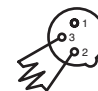
Termination reduces signal errors and avoids signal transmission problems and interference. It is always advisable to connect a DMX terminal, (Resistance 120 Ohm 1/4 W) between PIN 2 (DMX-) and PIN 3 (DMX +) of the last fixture.
