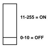
If the value of channel A is set between 0 to 10, the unit is off. While the value is set between 11 to 255, the unit is on.
