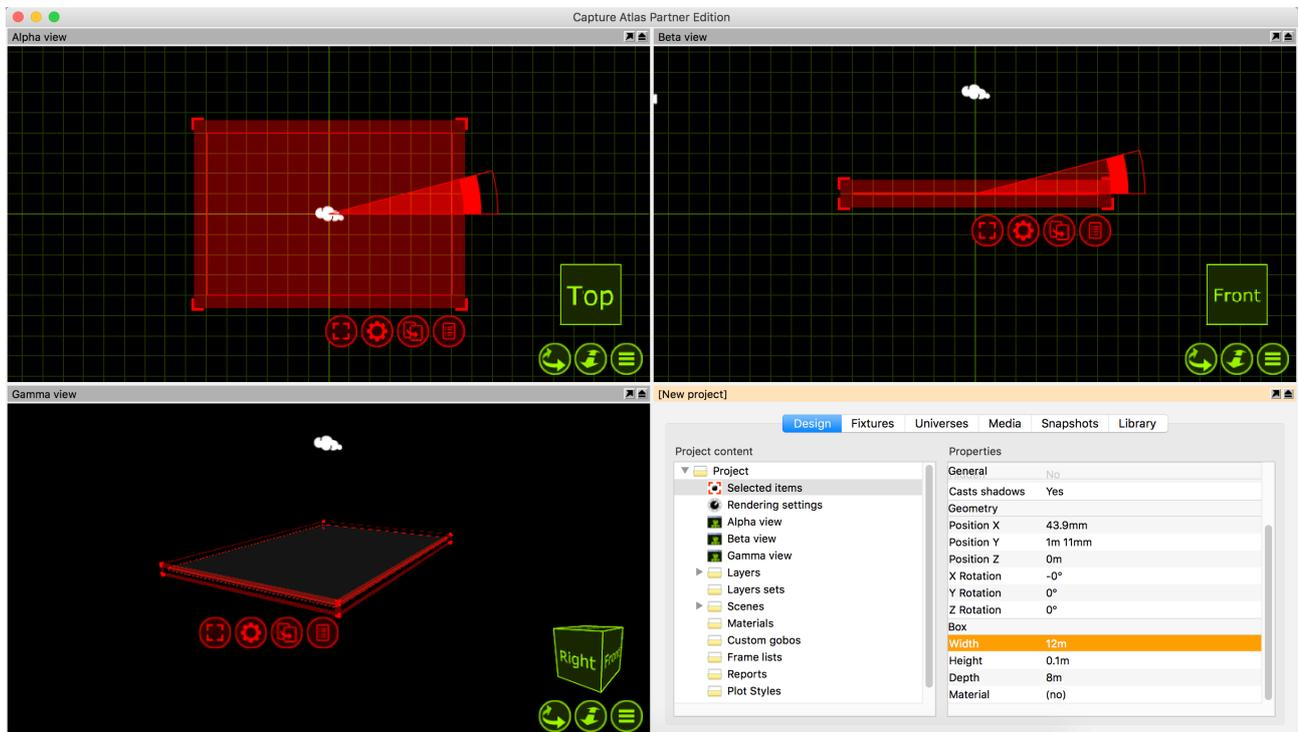
some more objects. We will add some truss in above the stage. Adding a piece of truss is done in the same way the box was added. Locate the desired piece in the library and drag it into either the Alpha or Beta view. For the sake of example, we will use a piece of truss from the **Generic** folder. Double click the **Truss** folder, double click again on the **Generic** folder, and again on **Box**. Choose the **Generic Rectangular Section** and drag it into one of the views.
