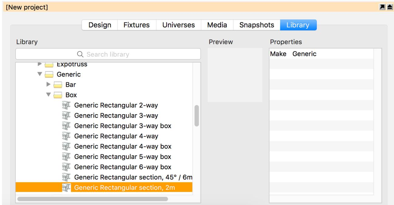
wide. We now want to add more 2m sections of truss to result in one long truss going from one side of the stage to the other. This can easily be done with the **Clone** feature.
