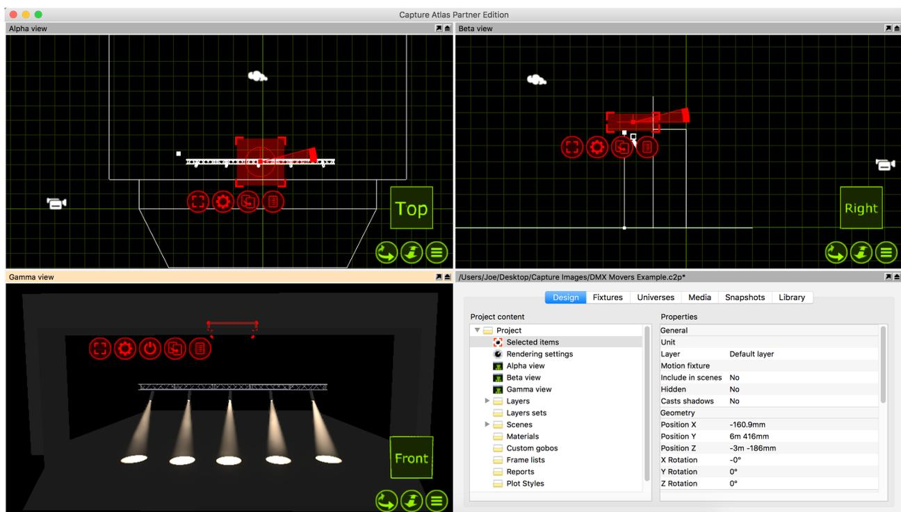
Select the Truss and the Fixtures you wish to rotate and select the DMX Rotator from the “Motion Fixture” property in the Project Window.
