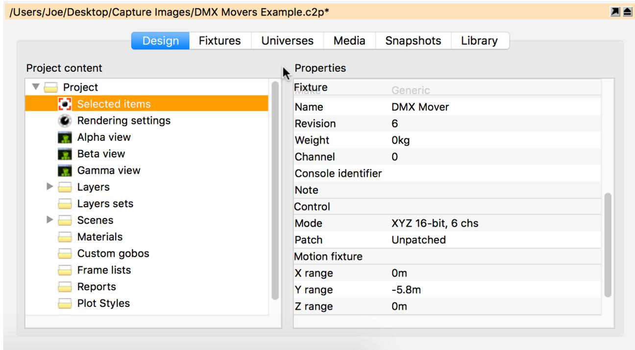
Select the Truss and the Fixtures you wish to move and select the DMX Mover from the “Motion Fixture” property in the Project Window.
