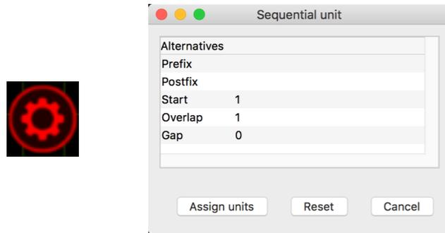
Sequential circuit essentially works just like sequential uniting – except that you assign circuit numbers to the Channel property of fixtures. You may specify a Prefix as well as a Postfix to the numbering.
