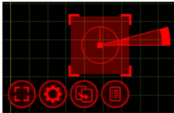
The DMX Rotator, pictured to the left, is shown here as it is seen in the "Orthographic Front" simulator view. The thick blob in the middle of the circle indicates the central rotation point that the object will rotate around. The line protruding from the centre of the circle from the blob is the default starting point. The circle itself indicates the range in which the Rotator can operate. In this case, it is a full circle as the Rotator has a range of 360 degrees.
