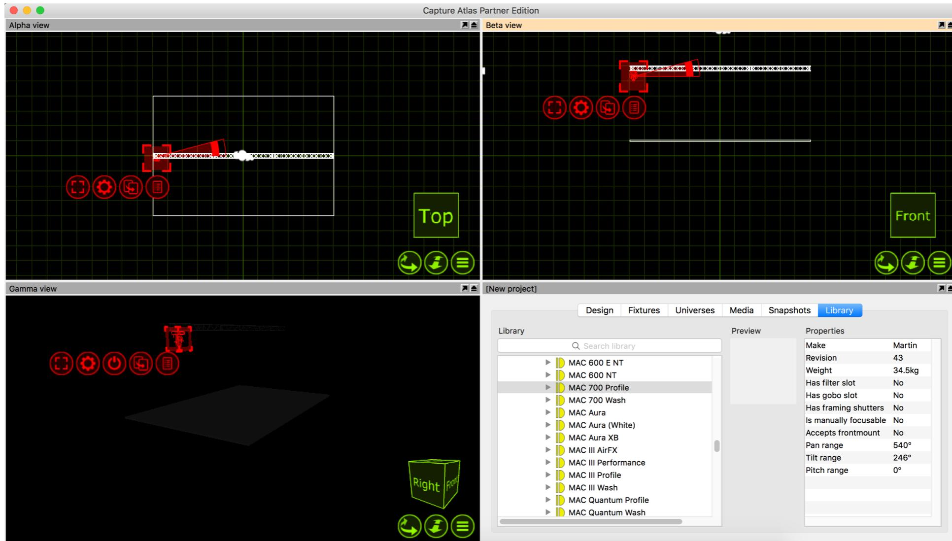
Clone the Mac 700 Profile 11 times so the 12m truss has 1 Mac 700 every meter.
