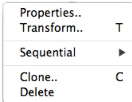
The second button is another options button, but in this instance, pressing it displays a small list of possible operations relevant to the selected object(s). The list that appears is context sensitive, that is to say that selecting a Lighting Fixture will display different options in the list than that of a Truss. Each available option/command will be covered later in the relevant chapters.
