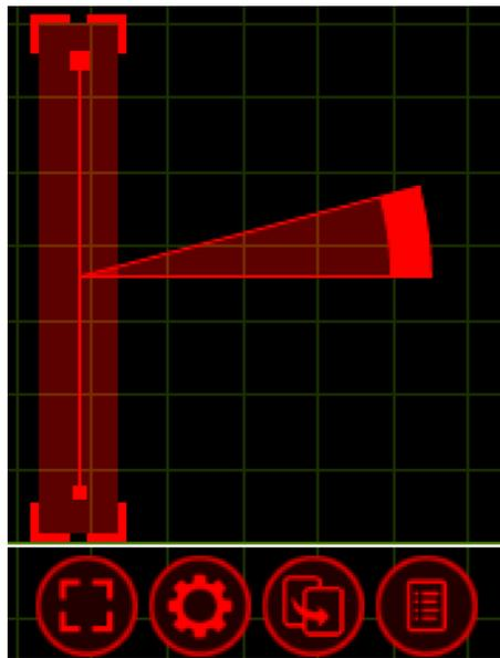
The DMX Mover, pictured to the left, has two blobs at each end of the range. The thicker blob indicates the default starting point of the object the Mover is attached to. The thinner blob indicates the lowest point to Mover operates to.
