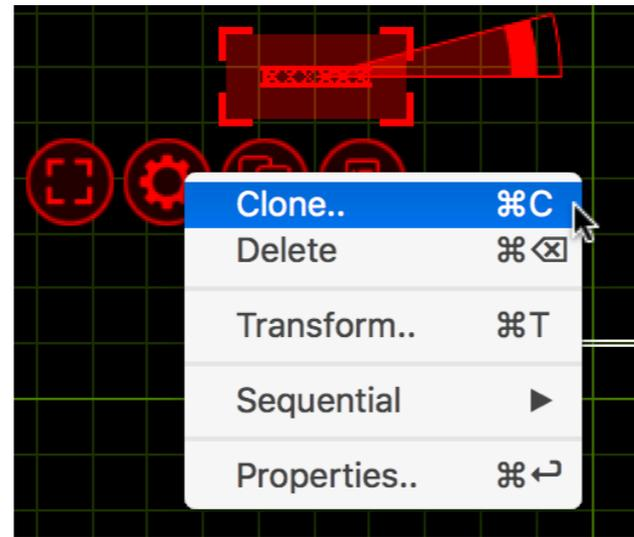
Click the **Clone** option, this will bring up the **Clone** window. Set the **X Offset** to **2m** and set the number of clones to **5**. This will then add sections of 2m truss right across our 12m wide stage evenly.
