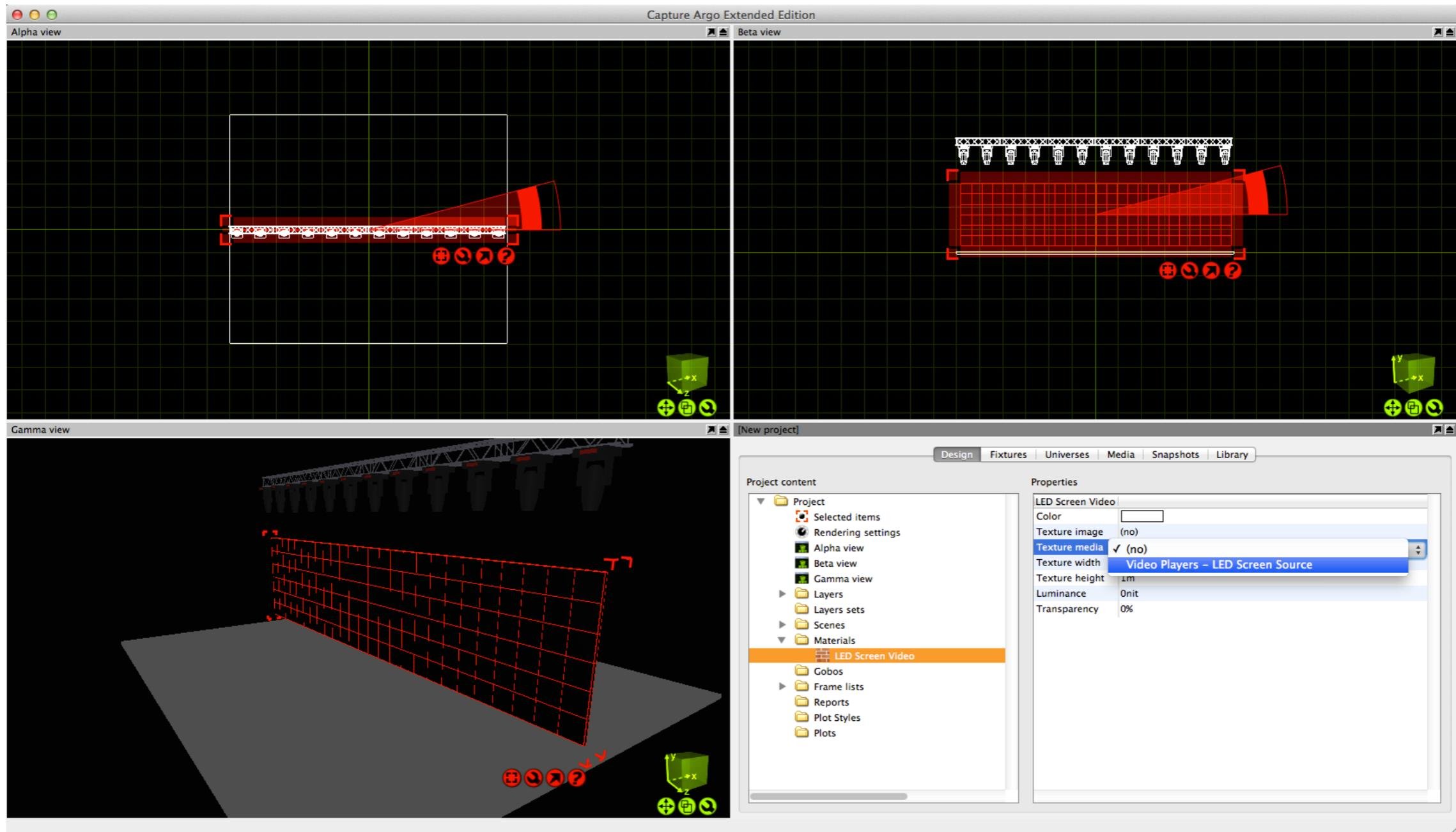
Once the Material has been assigned to the video player, drag the material from the project window to the LED Screen in one of the simulator views. Press the red spanner button and choose the "Map Material" option. Then select the "Map to extents" option, this will set the material to fill the whole screen.
