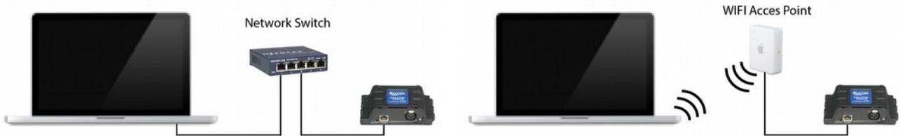
Per factory default the Touch is set DHCP. It will be automatically assigned with an IP address by the DHCP server in your network (usually done by your router). When set to DHCP the heartbeat LED on the Touch indicates red.
