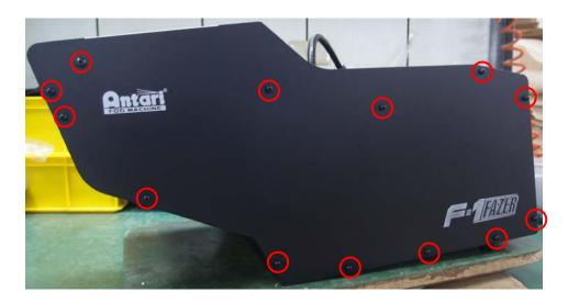
Step 2. Remove the screws on the side of F-1.
